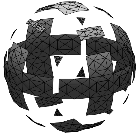
Figure 3: Area A_m(ct) which results from the intersection of the surface of a sphere with the radius ct = 10 m and all image source rooms with an order of 3 or less for a room geometry of 4.7 \times 4.2 \times 3.2 m 3 . The ratio of the intersection surface area and the sphere surface area yields the fade-in function f(t) = \sqrt{1 - \frac{A_m(ct)}{A(ct)}} for the late reverberation tail h(t) .
